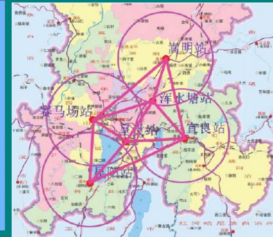
Kunming GPS Reference Station Network
